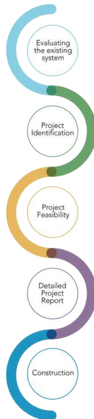
Figure 9: Phases required for setting up decentralized wastewater management systems (MoUD, 2012)
