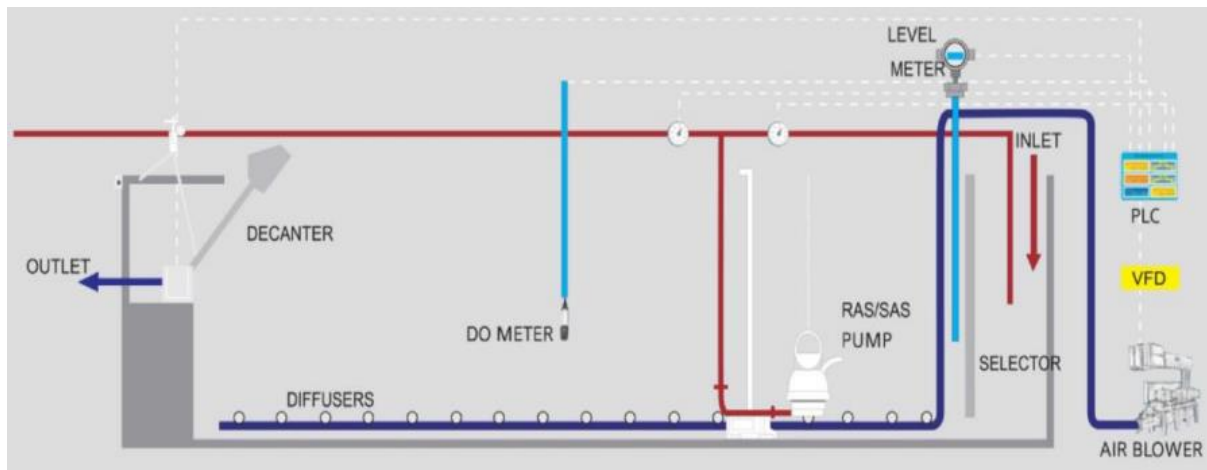
Figure 6: Component of C-Tech SBR System
