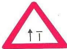
Lane Closed (Two Lane Road)
